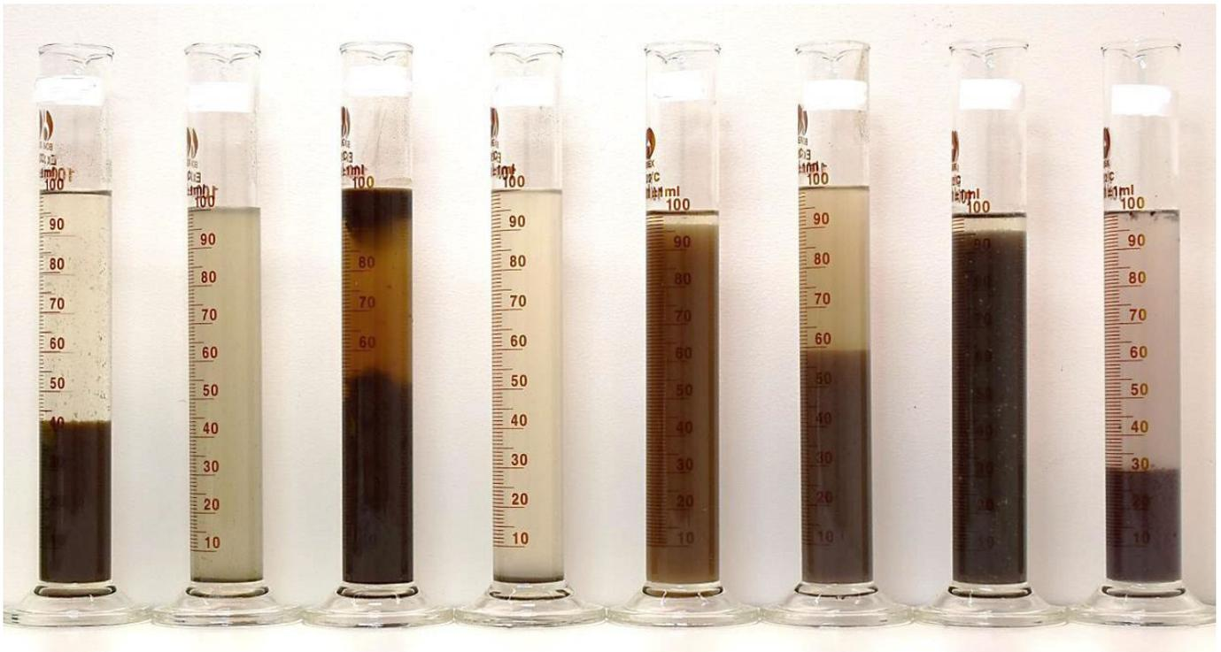
Figure 2. Sludge volume differences between wastewater treatment plants.
