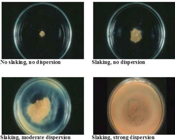
Figure 4: Assessment of an undisturbed soil aggregate after it has been placed in distilled water for a period of two hours. The higher the dispersion, the higher the sodicity. (Photo: Alf Cass).
