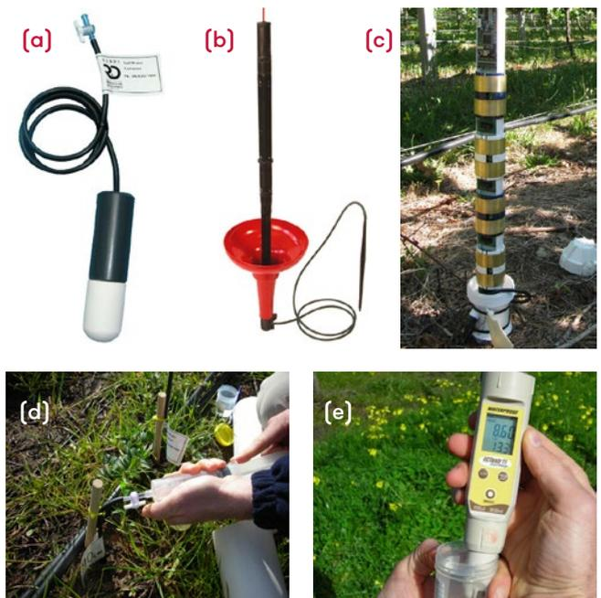
**Figure 3:** Examples of (a) a suction cup sampler, (b) a wetting front detector, and (c) a capacitance sensor. (d) Extracting soil water samples with a syringe, (e) testing a water sample with a handheld salinity meter. (Photos: SARDI, CSIRO & Sentek Technologies)
