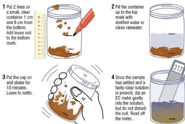
Figure 2: In-field assessment of soil salinity using a 1:5 soil-to-water extract (Source: Lanyon 2011).
