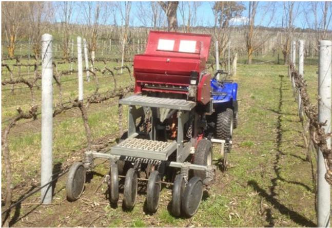
Fig 4. A Taeye disc seeder sowing one row either side of the vine.
