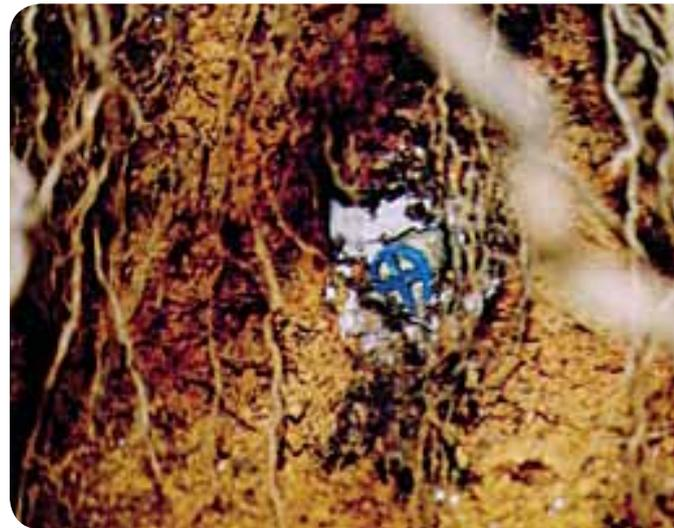
PHOTO 8: GYPSUM BLOCK POSITIONED WITHIN THE ROOTZONE
