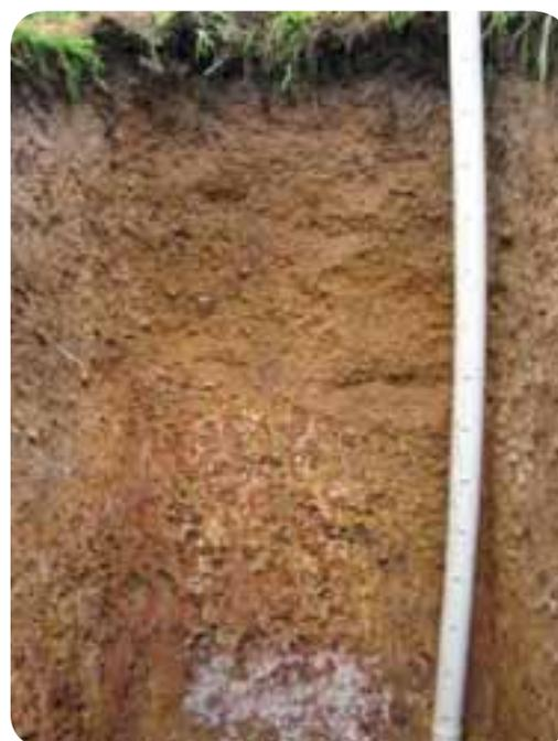
**PHOTO 1: TYPICAL GRAVEL SOIL PROFILE**
